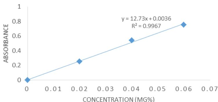
**Fig. 2: Calibration curve of Rabeprazole in SGF, pH 1.2 at 207nm**
