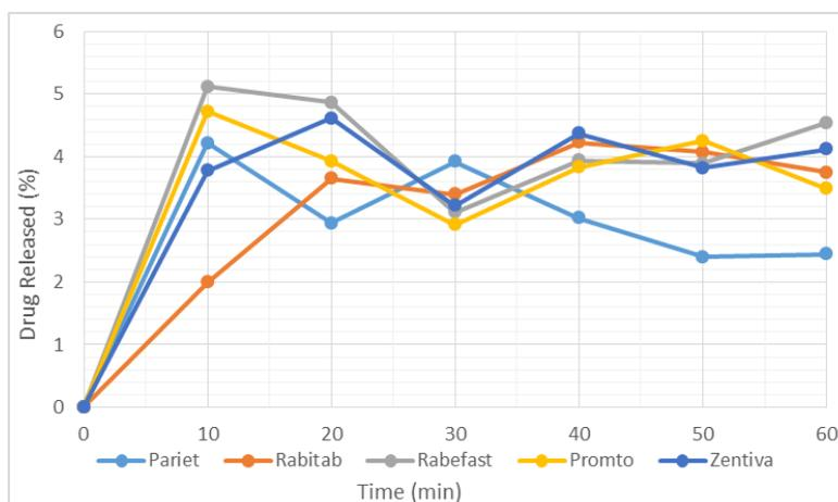
**Fig. 4: Graph of dissolution profile for the various brands of rabeprazole in SGF, pH 1.2 at 207nm**
