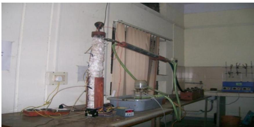
**Fig.1: Experimental set up of pyrolysis reactor**
